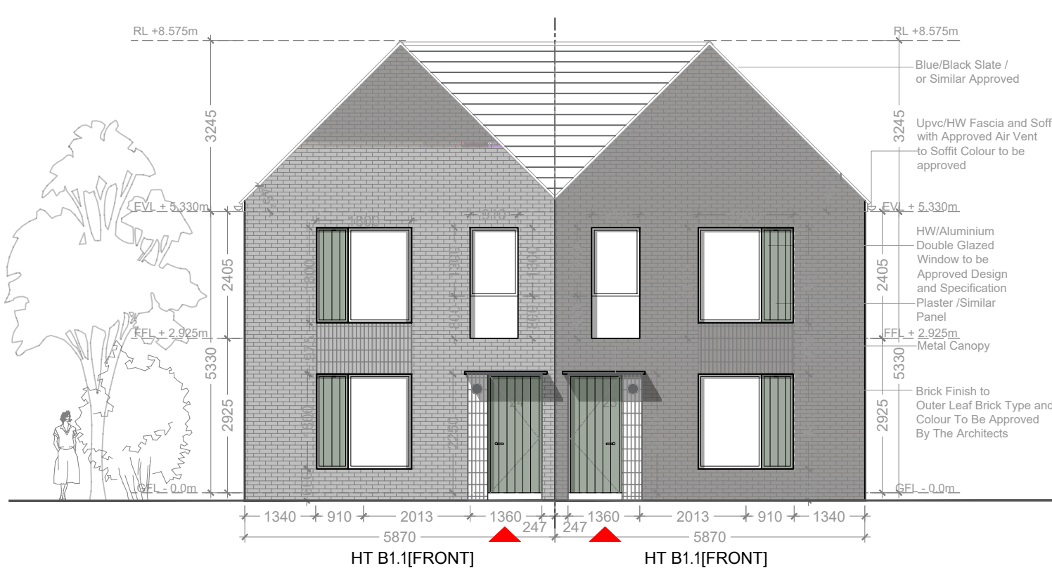
05 102 FRONT ELEVATION 1:100 BLOCKS 6&9
